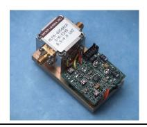
The CA series of analog driver provide the main coil current from the +15 volt input line. Current increases linearly from 0 mA = 0 GHz at a rate of approximately 50 mA per 1 GHz. A 2-8 GHz filter will require 100 mA @ 2 GHz and 400 mA @ 8 GHz.
